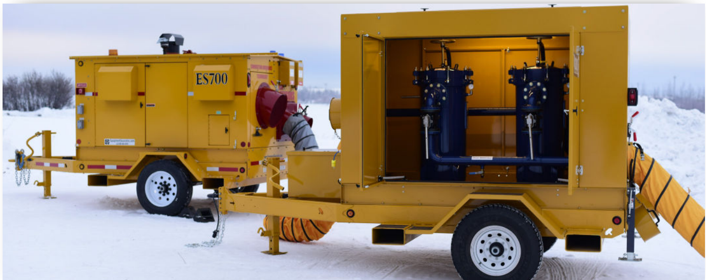
Clean, dry, safe hot air from an ESI heater heats the Filter Trailer enclosure and provides heated ducts through which product piping is routed
