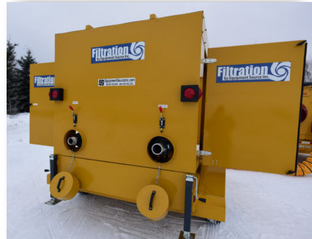
Duct covers keep snow and dirt out of the enclosure
