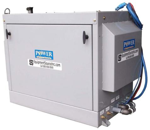
The APU-B by ESI is a 6 kilowatt portable diesel generator set with a heat exchanger system. The heat exchanger system transfers heat through coolant to another circuit such as a truck engine. The secondary coolant circuit has integrated quick disconnects and a circulation pump to maintain coolant flow. In addition to providing heat, the unit also provides AC power for auxiliary use.
