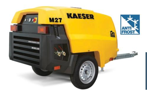
Our unique anti-frost valve maintains optimal air temperature to prevent ambient moisture from freezing in air tools.
