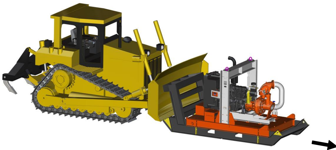
Figure 12: Pushing Typical Large Pumpset Unit
