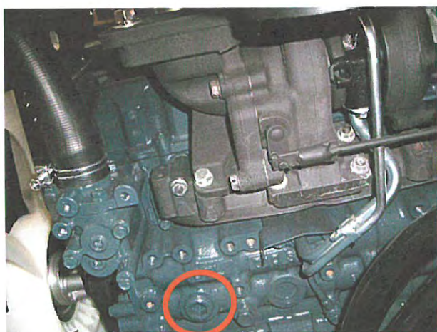
Step.3. Locate the plug on the right side of the engine.
