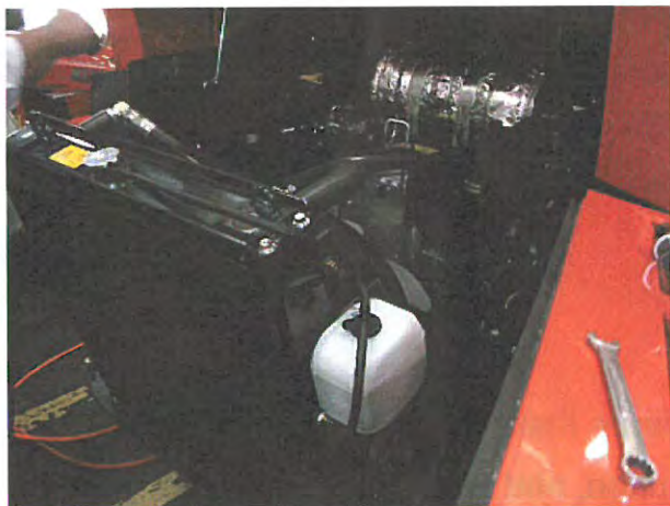
Step.1. Slide out and tilt the radiator after removing the (4) 19mm mounting bolts. Secure using the radiator in place.
